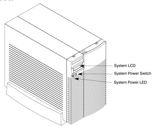
Figure 1–1. System Unit Front Panel Controls
