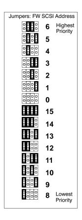
Figure A–15. Fast, Wide Hard Drive Jumper Settings
