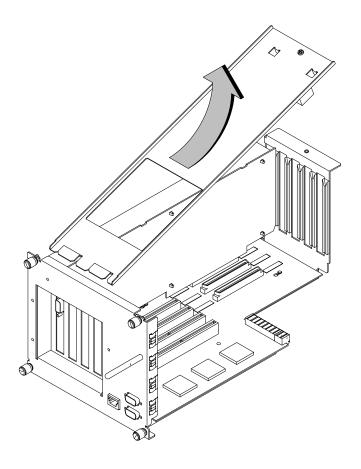
Figure A-34. Removing the EISA Assembly Cover
