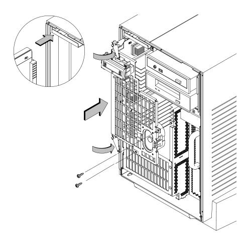
Figure A-24. Replacing the CPU Assembly
