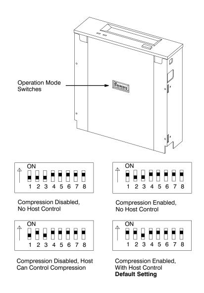
Figure A–9. Switch Settings for Data Compression Operation Mode
