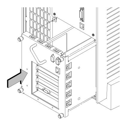
Figure A-39. Replacing EISA Assembly
