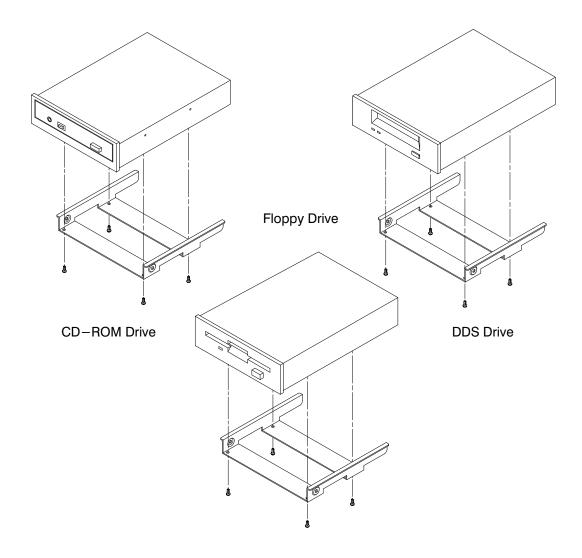
Figure A-12. Attaching Removable Drive Mounting Bracket and Drive Orientation
