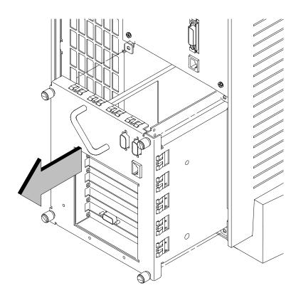
Figure A-32. Removing the EISA Assembly
