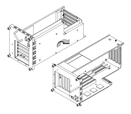
Figure A–33. Rotating the EISA Assembly for Installation
