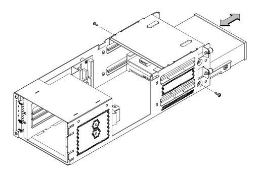
Figure A–5. Removing Drive Screws
