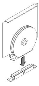
Figure A-28. Removing CPU and Connector Dust Covers
