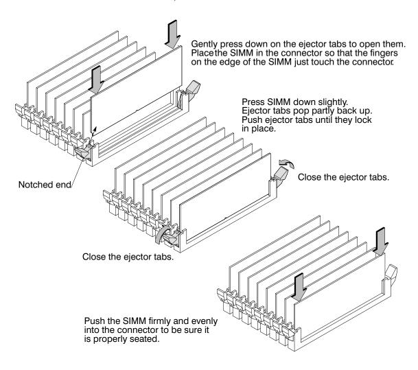
Figure A-23. Installing Memory Cards
