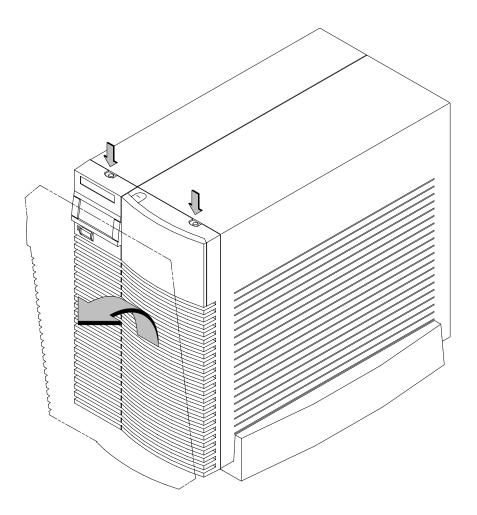
Figure A-1. Removing the Front Panel
