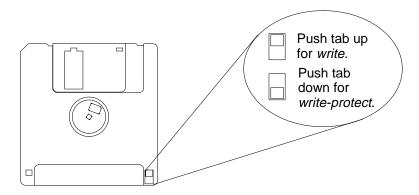
Figure 5–1. Setting the Write-Protect Tab on a Floppy Diskette
