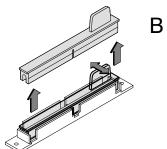
3. Install the processor module into the connector by lining it up over the connector and pressing firmly and evenly.
