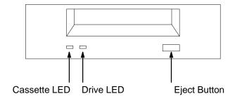
Figure 5–1. DDS Drive Controls and Indicators
