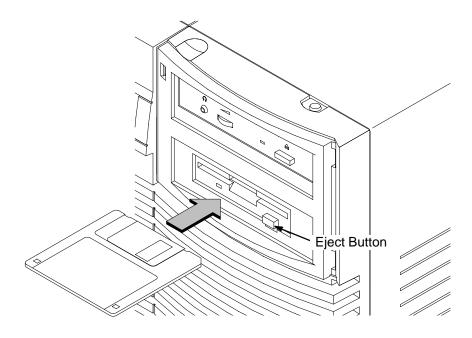
Figure 5–2. Inserting and Removing a Floppy Diskette
