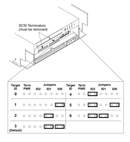
Figure A-7. DDS-DC Tape Drive SCSI Address/Jumper Settings
