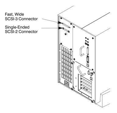
Figure C-2. Rear Panel SCSI Connectors without Terminators
