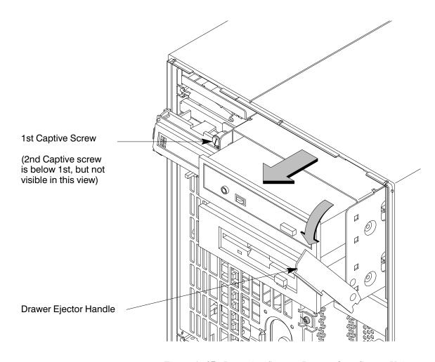
Figure A-17. Removing Storage Drawer from System Unit
