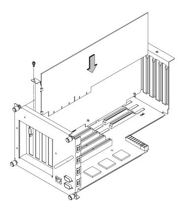
Figure A–36. Installing an EISA or Graphics Board in the EISA Assembly
