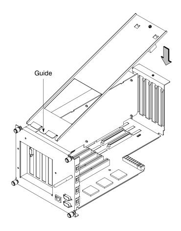
Figure A-37. Replacing EISA Assembly Cover
