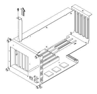
Figure A-35. Removing the EISA Slot Cover
