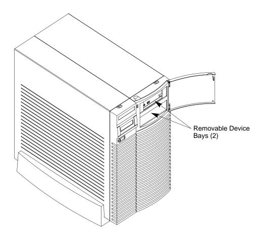
Figure 1–3. System Unit with Removable Device Door Open
