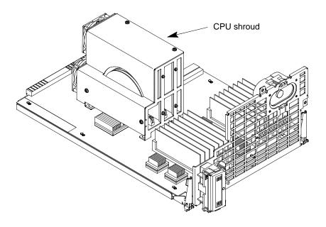
Figure A-26. CPU Shroud Location
