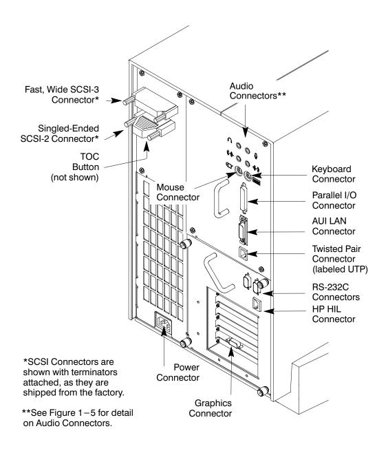
Figure 1-4. System Unit Rear Panel Connectors
