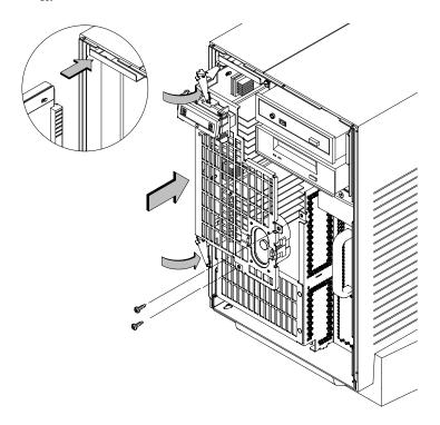
Figure A-29. Replacing the CPU Assembly
