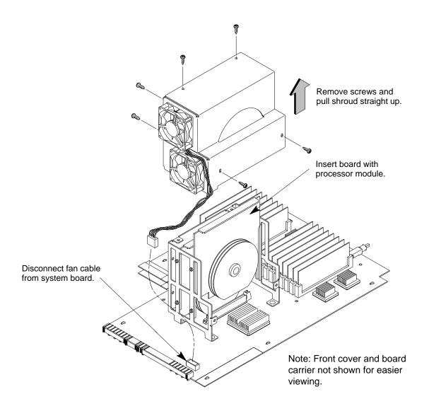
Figure A-27. Removing CPU Shroud and Disconnecting Fan Cable
