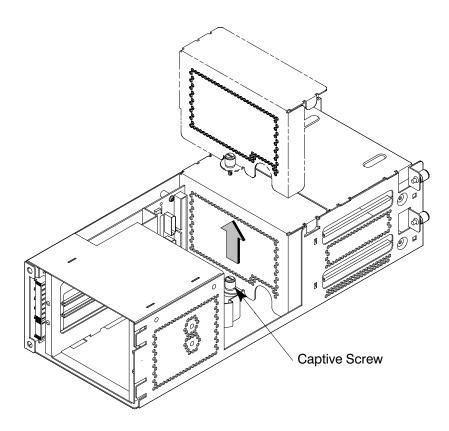
Figure A-4. Removing EMI Plate
