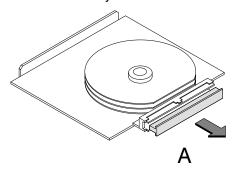
To remove the dust cover on the CPU board, grasp the tab on the right side of the cover and gently rock the cover back and forth while pulling it gently up.
