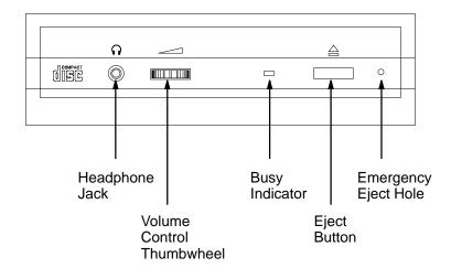
Figure 6–1. CD-ROM Drive Controls and Features
