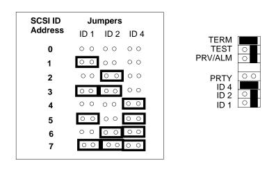
Figure A-6. CD-ROM Drive SCSI Address/Jumper Settings
