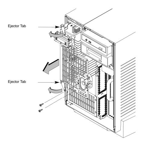
Figure A-19. Removing the CPU Assembly
