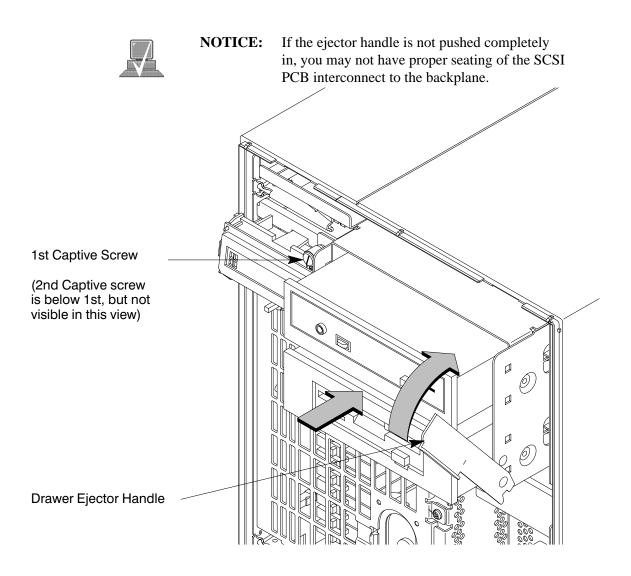
Figure A-14. Replacing the Storage Drawer Assembly
