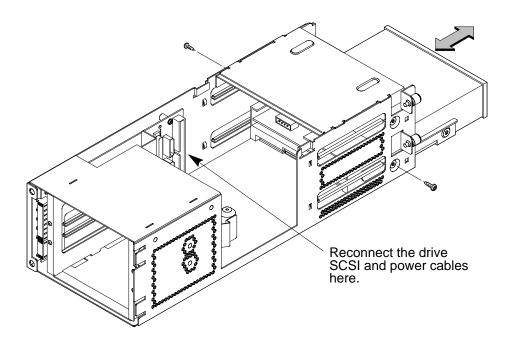
Figure A–13. Replacing Drive Screws
