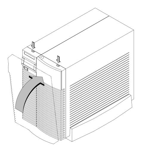
Figure A-2. Replacing the Front Panel
