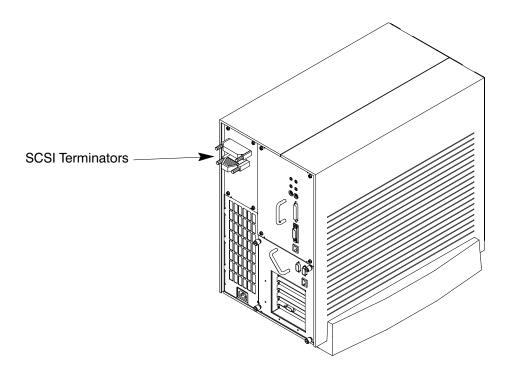
Figure C-1. Rear Panel SCSI Connectors with Terminators Attached
