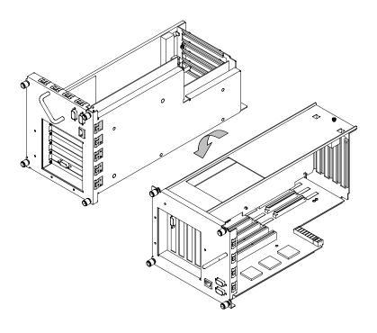
Figure A-38. Rotating the EISA Assembly Back
