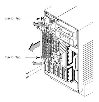
Figure A-25. Removing the CPU Assembly
