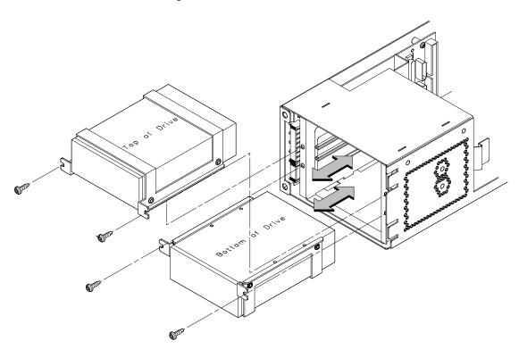
Figure A-18. Placing Hard Drives in Storage Drawer
