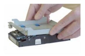
4. Insert the T-15 Torx Hard Disk Mounting Screws through the rubber mounting grommets and into the screw holes located on the sides of the hard disk drive. See Figure 4-40.
